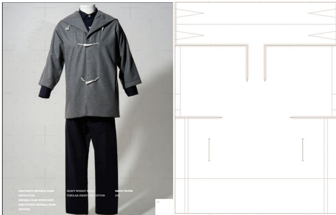
Image 5: Minimum seam duffle coat, work shirt and trousers, along with the zero waste pattern designed to create them, created by David Telfar in 2010 and shown in the Yield exhibition (McQuillan & Rissanen, 2011).
